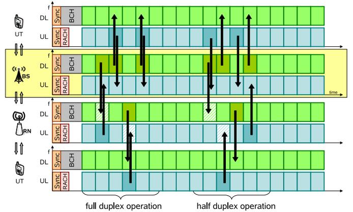
Fig. 2. FDD full and half duplex for 3GPP-LTE [7]
