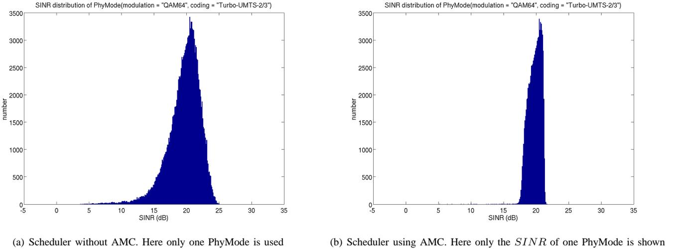
Fig. 10. probability density functions of the SINR at the receiver with and without Adaptive Modulation and Coding
