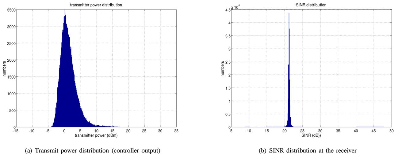
Fig. 11. Using Adaptive Power Control (APC) in DL: Transmitted and received power probability density functions
