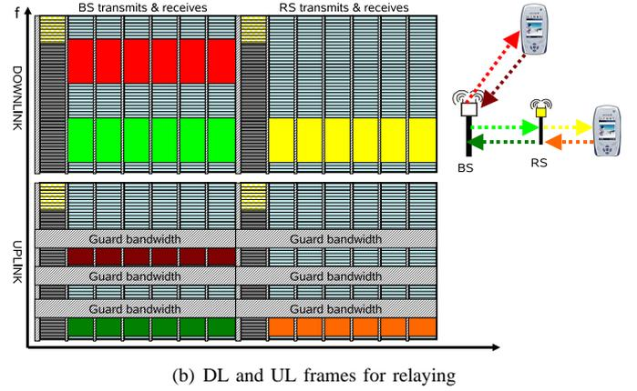
Fig. 1. Left: TTI Frame format for 3GPP-LTE [6] ( $500\mu s$ ). Right: Resource allocation for two hops.
