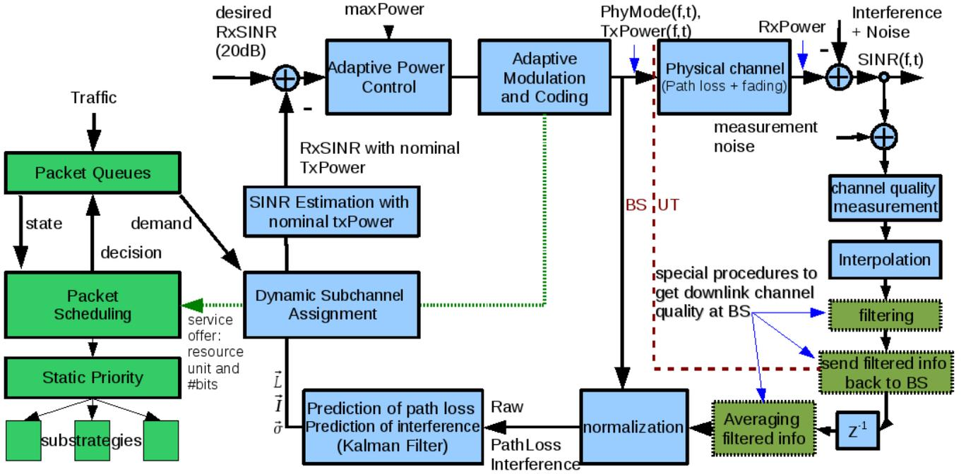
Fig. 1. Closed Loop Control view of the OFDMA DL resource scheduling tasks. The desired  $SINR$  at the receiver is sufficient to support the highest possible LTE PhyMode. The packet scheduling tasks are shown in green to the left.
