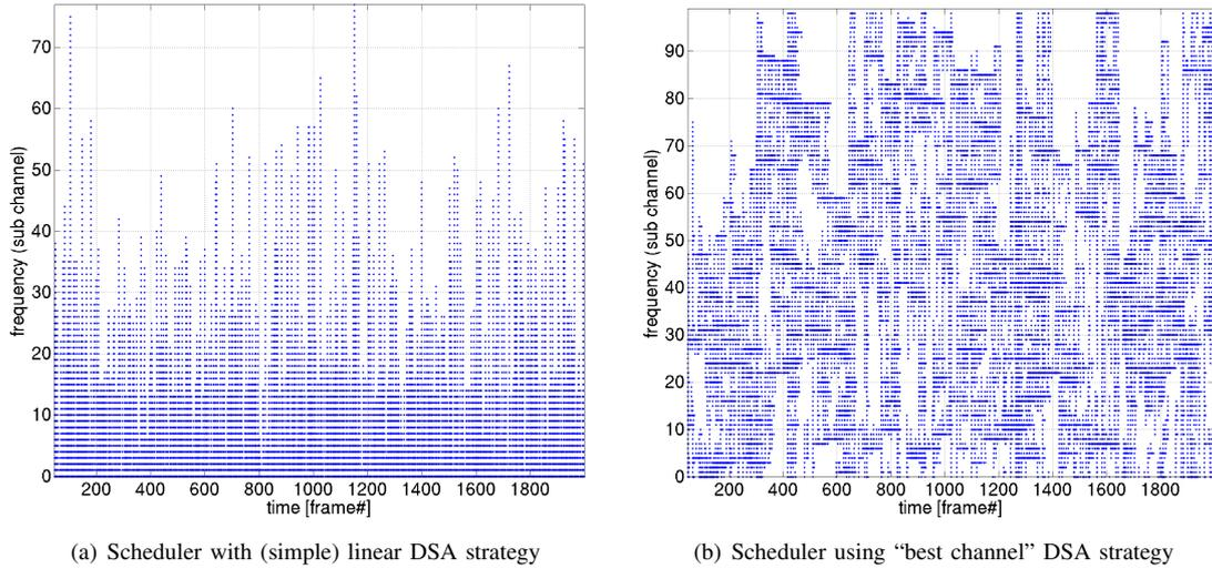
Fig. 2. Used DL resources in time and frequency with Dynamic Subcarrier Assignment strategies LinearFF and BestChannel. Distance = 768m.
