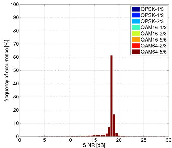
(a) Actual transmit power distribution using APC (controller output). The nominal power would be  $26\text{dBm}$  per subchannel. (b) SINR distribution at the receiver when APC is applied. Compare with Fig. 5.
