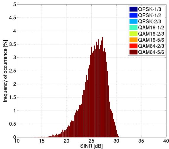
Fig. 5. SINR at the receiver without Adaptive Power Control (APC) at a distance =  $768\text{m}$ .
